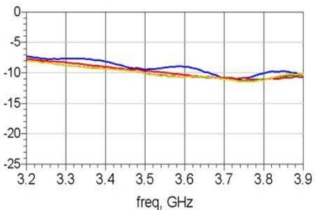
Figure 11.1.3: S12(Rev Iso) vs Freq
