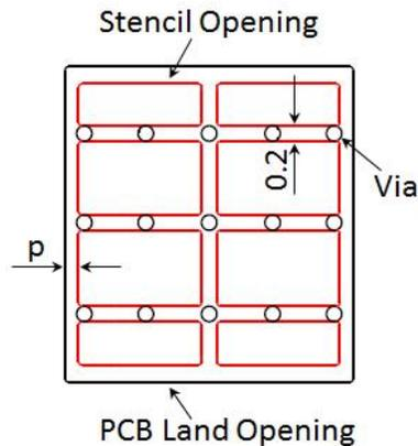
**Figure 15.2 Stencil Openings Shall Not Cover Via Areas If Possible**
