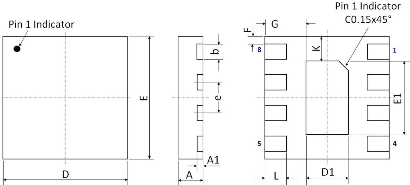
**Figure 13.1 Device Package Drawing**
