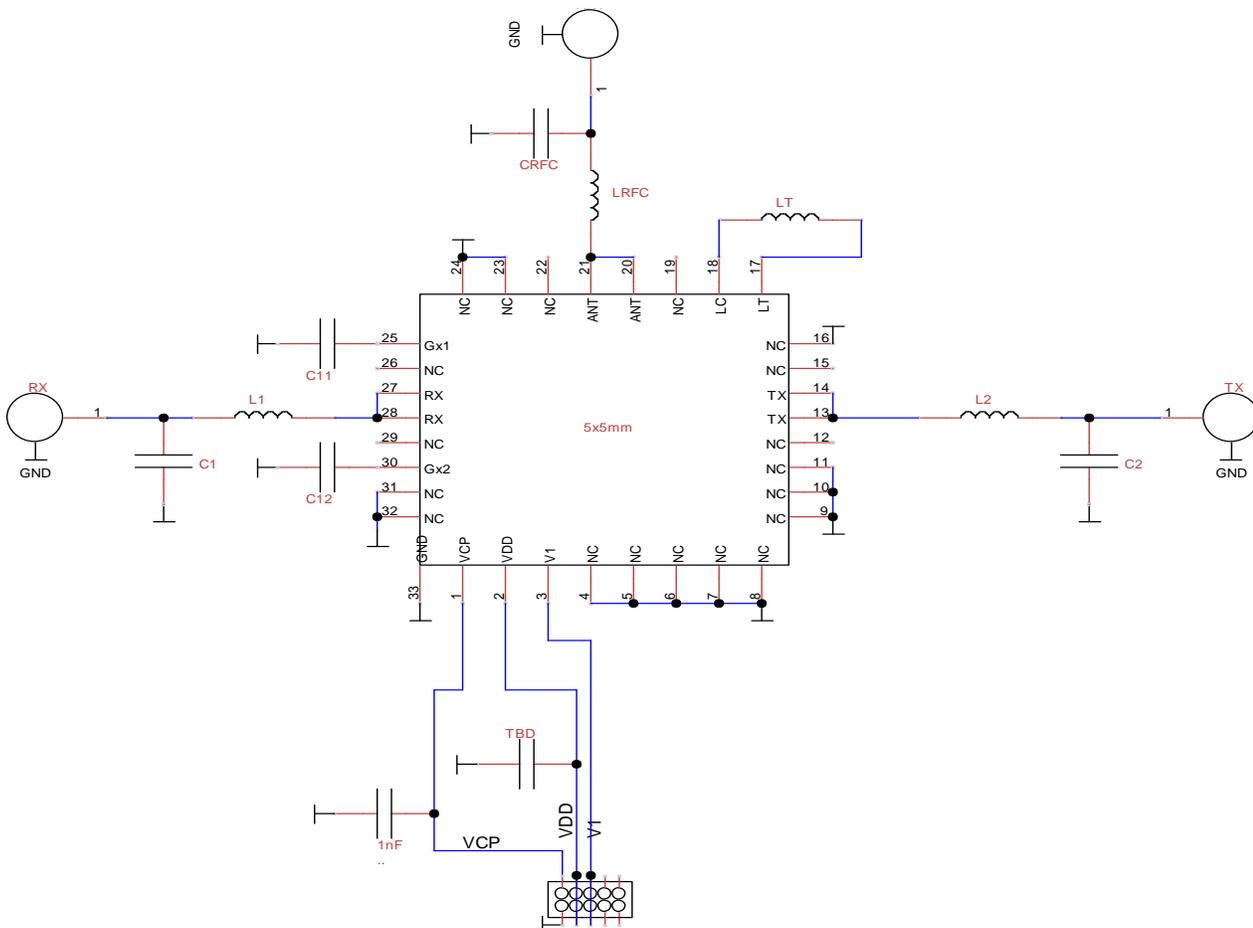
**Figure 3 Evaluation Board Schematic**
