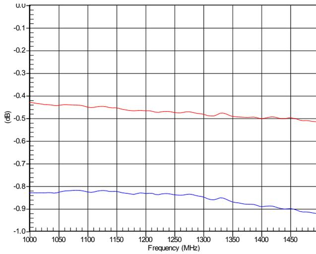
**Figure 4 TX (Red), RX (Blue) Insertion Loss**
