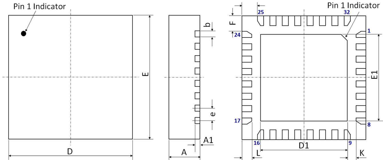
**Figure 12 Device Package Drawing**
