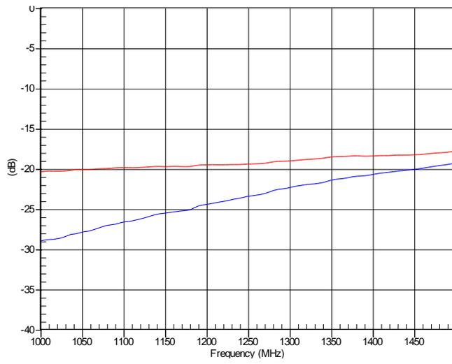
**Figure 7 TX (Red), RX (Blue) ANT Return Loss**
