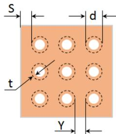
**Figure 15 Thermal Via Pattern**
