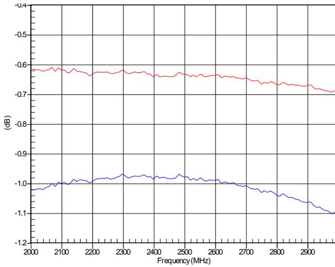
**Figure 8 TX (Red), RX (Blue) Insertion Loss**
