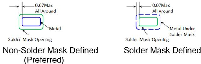
**Figure 14 Solder Mask Pattern**
